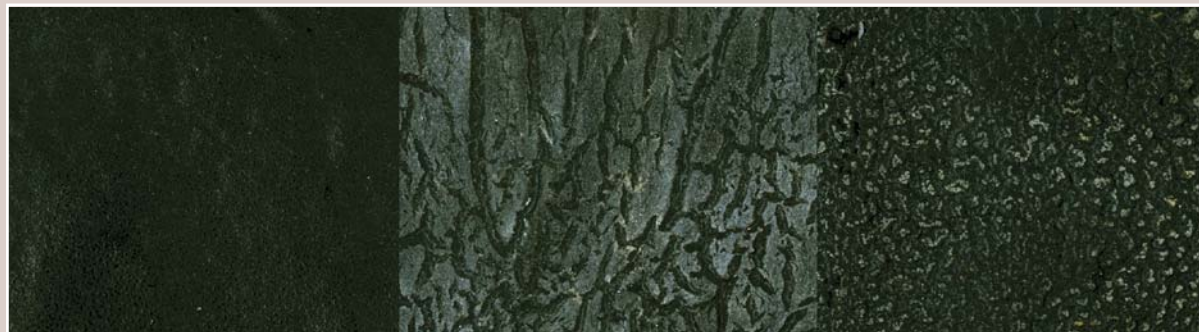
Here's dramatic proof . . . unretouched photos of Heavy Duty Patching Compound (left) and two leading competitors (middle & right) after a 1,000 hour accelerated weathering test. Notice varying degrees of oxidation of the competitors and lack of oxidation on the SWEPCO sample. Which do you want on your roof?
